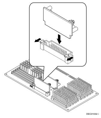
Figure 5-6. Installing a VRM
