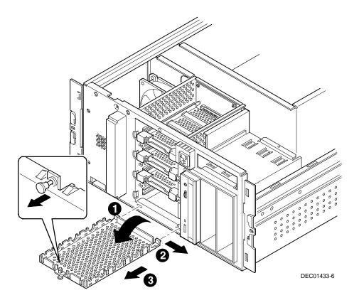
Figure 9-6. Removing the SCA-2 Drive Bay Cage Cover
