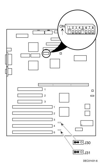
Figure A-1. Main Logic Board Switch and Jumper Locations
