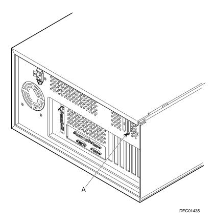
Figure 9-12. Connecting an External SCSI Device to a SCSI or RAID Adapter
