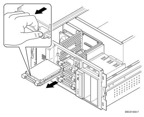
Figure 9-7. Removing the SCA-2 Disk Drive and SCA-2 Drive Tray
