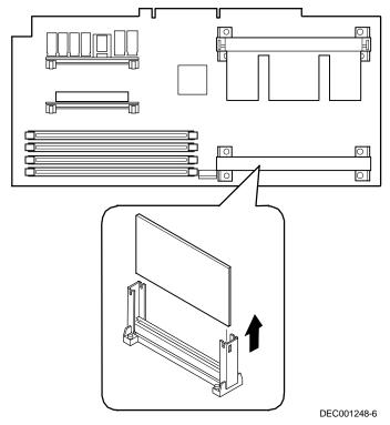
8. Remove the terminator card from the processor module slot (see Figure 6-2). Grasp the terminator by each end and pull up.
