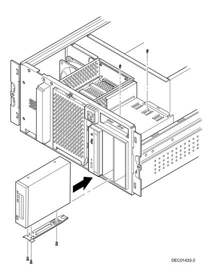
Figure 9-3. Installing a Half-Height 5<sup>1</sup>/<sub>4</sub>-Inch Device Into the Front Access Drive Bay
