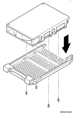
4. Remove the SCA-2 disk drive from the SCA-2 drive tray.
