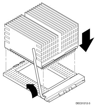
4. Lower the lever to engage the pins (Figure 5-4).
