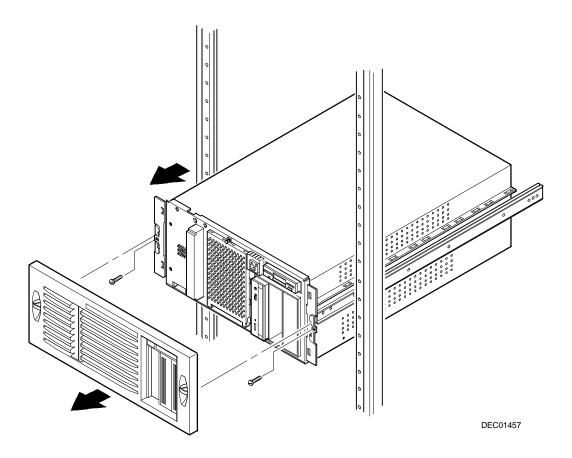
Figure 3-11. Removing the Front Bezel
