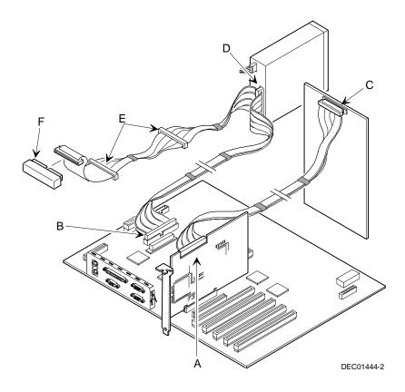
Figure 11-2. Single Channel RAID Configuration
