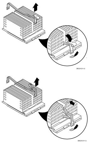
Figure 5-2. Removing the Retaining Clip
