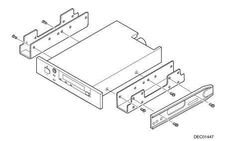
Figure 9-5. Installing 3<sup>1</sup>/<sub>2</sub>-Inch Expansion Brackets
