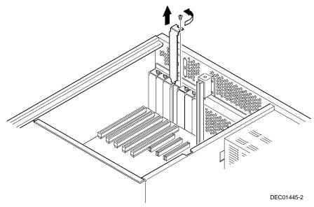
Figure 10-2. Removing a Metal Filler Plate
