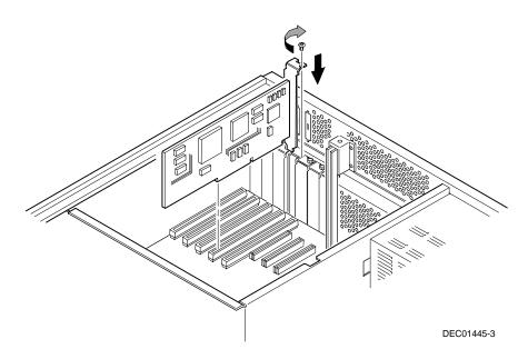
Figure 10-4. Installing an EISA Expansion Board
