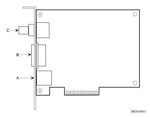
Figure 3-10. Ethernet Daughter Card Components and Connectors
