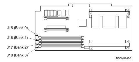
Figure 8-1. DIMM Socket Locations
