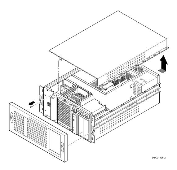
Figure 3-1. Removing the Top Cover
