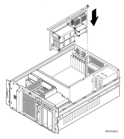
Figure 6-5. Installing the Pentium II Processor Module
