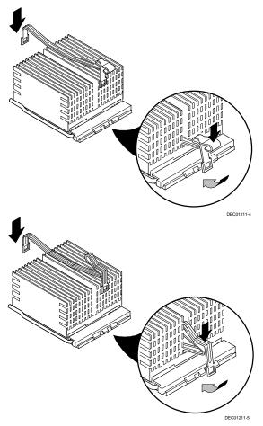
Figure 5-5. Installing the Retaining Clip
