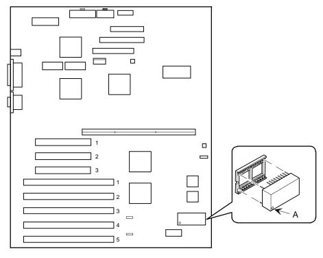
7. Remove the old battery/RTC (see Figure 3-12).
