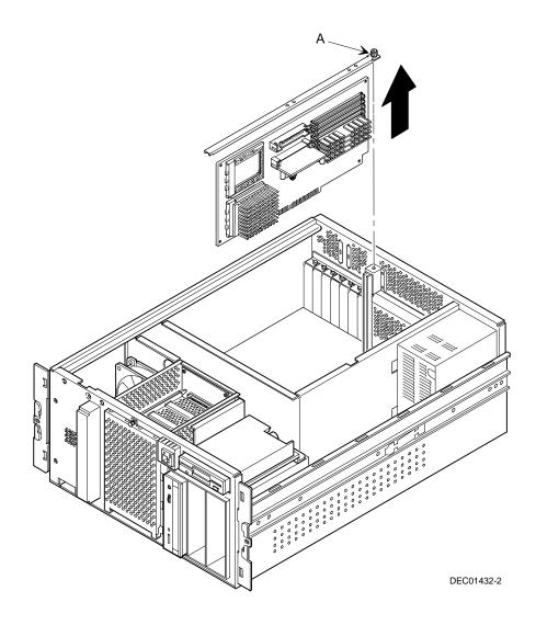
Figure 5-1. Removing the Processor Module
