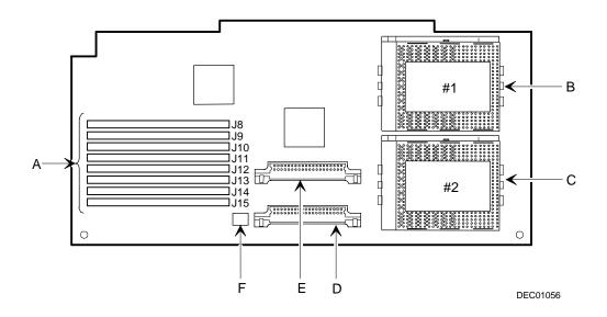
Figure 3-8. Pentium Pro Processor Module Components and Connectors
