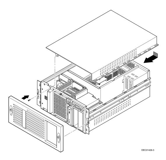
Figure 3-2. Installing the Top Cover
