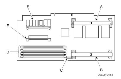
Figure 3-9. Pentium II Processor Module Components
