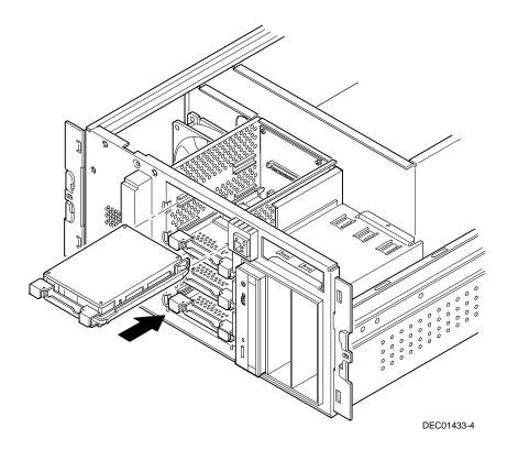
Figure 9-9. Installing an SCA-2 Disk Drive Into the SCA-2 Drive Bay
