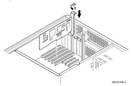
Figure 10-3. Installing an ISA Expansion Board
