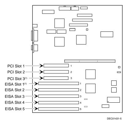
$^{(1)}\,$  PCI slot 3 and EISA slot 1 share an expansion slot at the rear of the server
