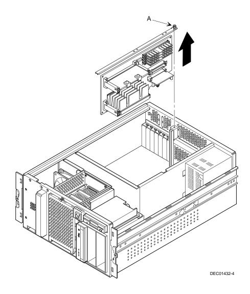
Figure 6-1. Removing the Processor Module
