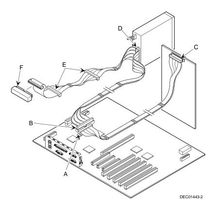
Figure 11-1. Wide and Narrow SCSI Cable Configurations
