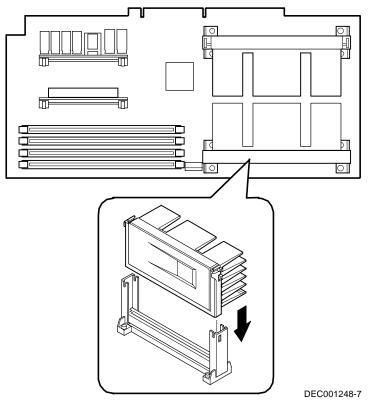
Figure 6-3. Installing the Second Processor
