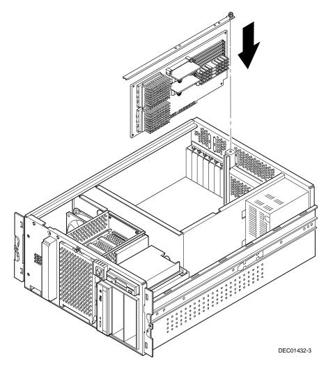
Figure 5-7. Installing the Processor Module
