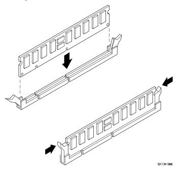
Figure 6-4. Installing a DIMM
