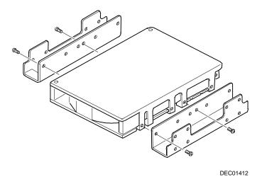
Figure 7-5. Installing Expansion Brackets
