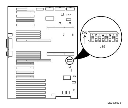
Figure A-1. Main Logic Board Switch Location
