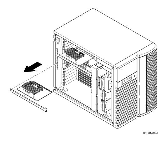
Figure 6-3. Removing a Memory Module
