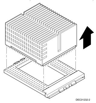
Figure 5-6. Removing the Processor/Heat Sink Assembly
