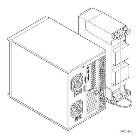
Figure 7-7. Connecting an External SCSI Device to a SCSI Adapter
