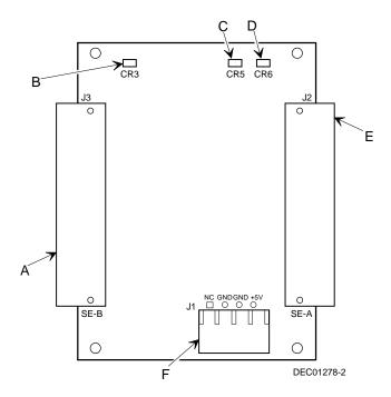
Figure 3-11. Wide Ultra SCSI Repeater Module Component Locations
