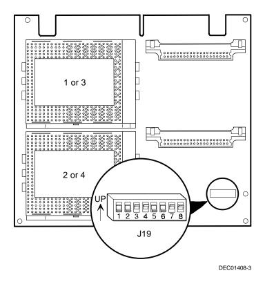
Figure A-2. Processor Module Switch Location
