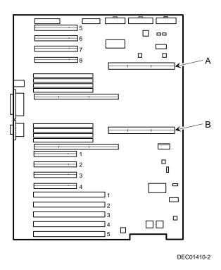
Figure 5-1. Processor Module Locations
