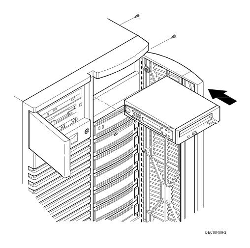
Figure 7-3. Installing a Half-Height 5¼-Inch Device Into Top-Right Drive Bay
