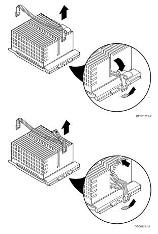
Figure 5-5. Removing the Retaining Clip
