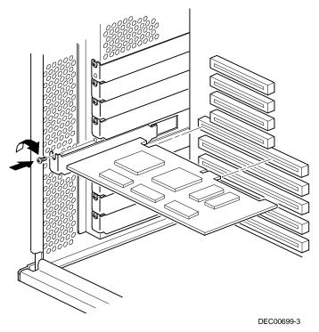
Figure 8-4. Installing an ISA Expansion Board
