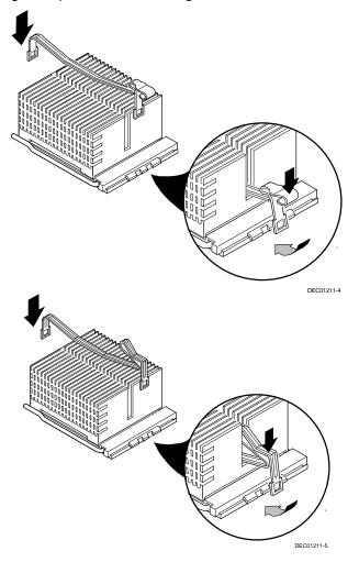
Figure 5-8. Installing the Retaining Clip
