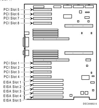
Figure 8-1. Expansion Board Slot Locations
