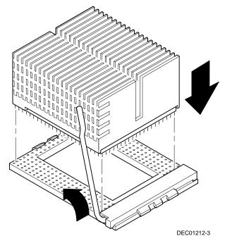
Figure 5-7. Installing the New Processor
