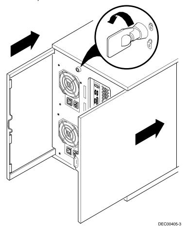
Figure 3-3. Installing Side Covers
