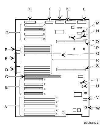
Figure 3-8. Main Logic Board Connectors
