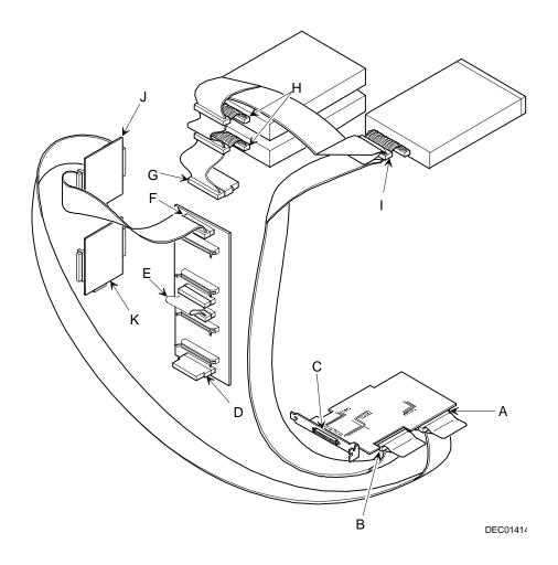
Figure 9-1. Single Backplane Configuration Using Two Channel SCSI Adapter
