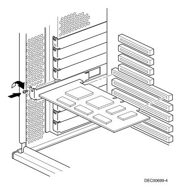
Figure 8-5. Installing an EISA Expansion Board
