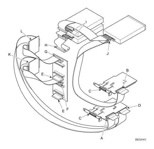
Figure 9-2. Split Backplane Configuration Using Two Channel SCSI or RAID Adapter
