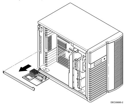
Figure 5-4. Removing the Processor Module
