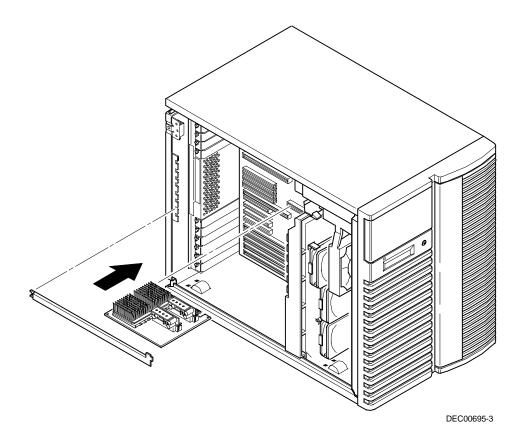
Figure 5-3. Installing a Processor Module
