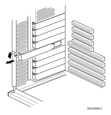
Figure 8-3. Removing a Metal Filler Plate
