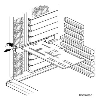
Figure 8-6. Installing a PCI Expansion Board
