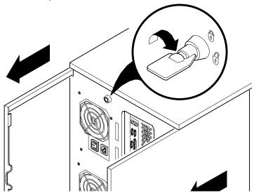
Figure 10-2. Left and Right Side Panel Lock
