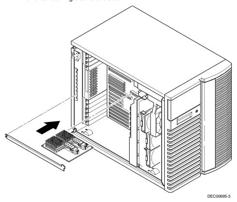
Figure 5-10. Installing the Processor Module
