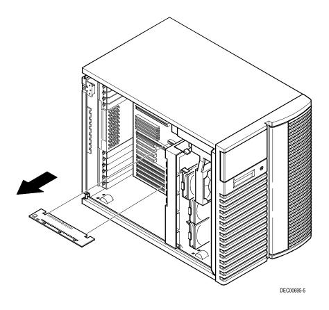
Figure 5-2. Removing the Terminator Card
