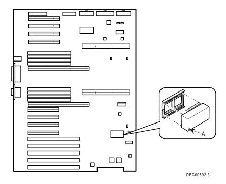
Figure 3-12. Replacing the Server Battery/RTC
