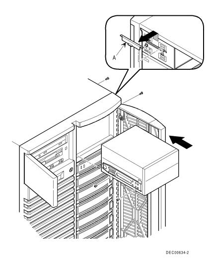
Figure 7-4. Installing a Full-Height 5¼-Inch Device Into Top-Right Drive Bay
