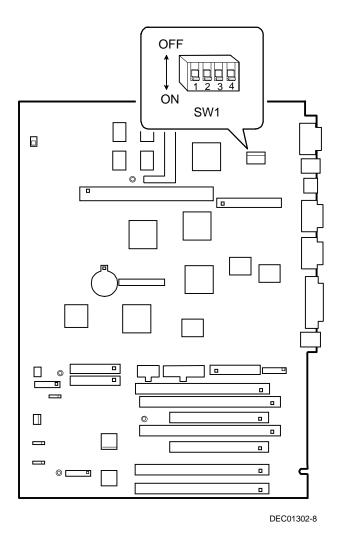
Figure A-1. Main Logic Board Switch Locations
