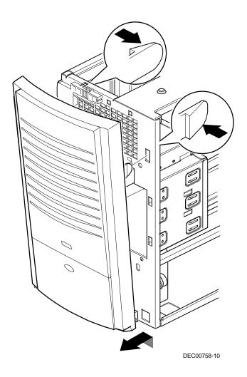
Figure 6-1. Removing the Front Bezel
