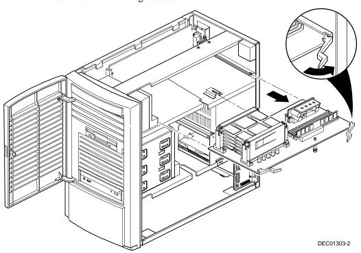
Figure 3-9. Removing the Pentium® II Processor Module
