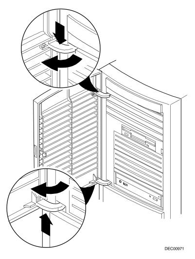
Figure 1-13. Removing the Front Bezel Door
