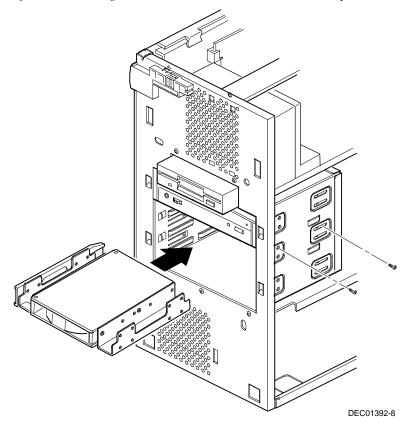
Figure 6-3. Installing a 3½-Inch Device
