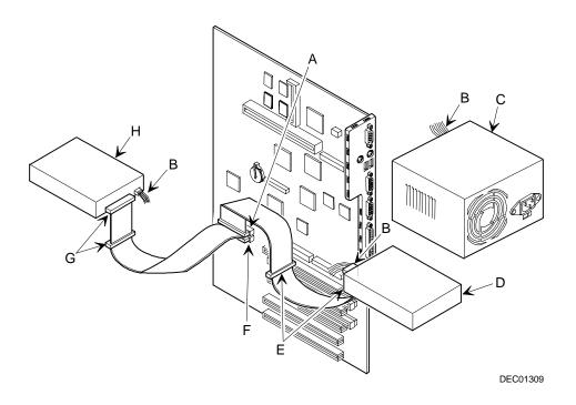
Figure 6-8. IDE Device Data Cable Connections
