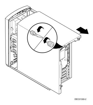
Figure 1-3. Removing the Outside Cover
