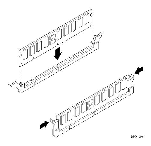
Figure 4-2. Installing a DIMM
