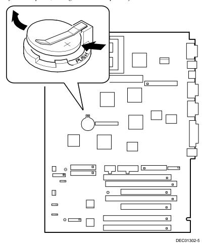
Figure 3-8. Replacing the Battery
