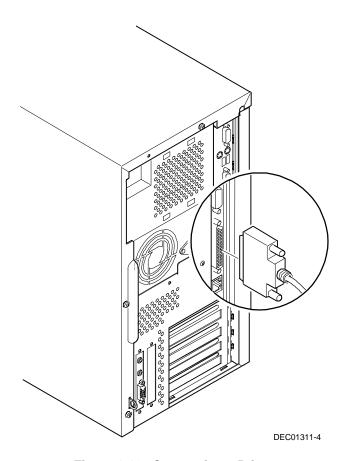
Figure 1-10. Connecting a Printer
