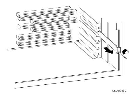
Figure 5-2. Removing a Metal Filler Plate
