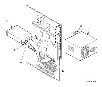
Figure 6-7. Diskette Device Data Cable Connections
