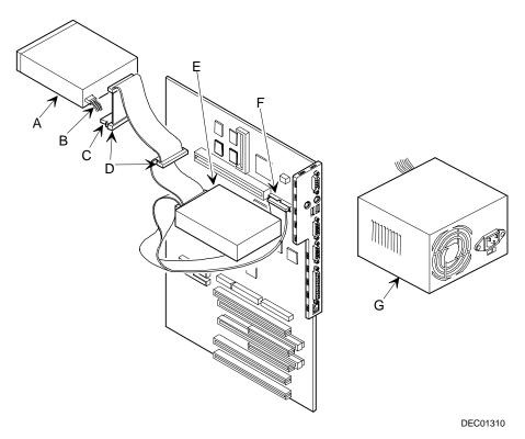
Figure 6-9. SCSI Device Data Cable Connections
