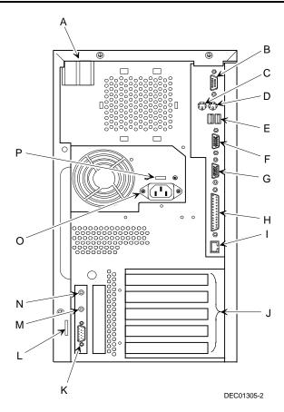
Figure 1-2. Rear Panel Connectors and Voltage Select Switch
