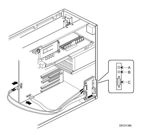
Figure 3-6. Audio/MIDI/Joystick Adapter Card Connectors
