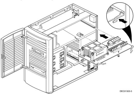
Figure 3-13. Replacing the Pentium® II Processor Module
