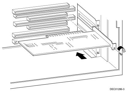
Figure 5-3. Installing an Expansion Board
