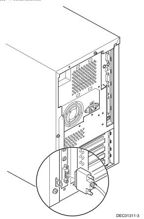
Figure 1-9. Connecting a MIDI/Joystick Device
