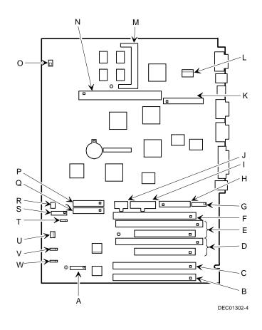
Figure 3-4. Main Logic Board Connectors
