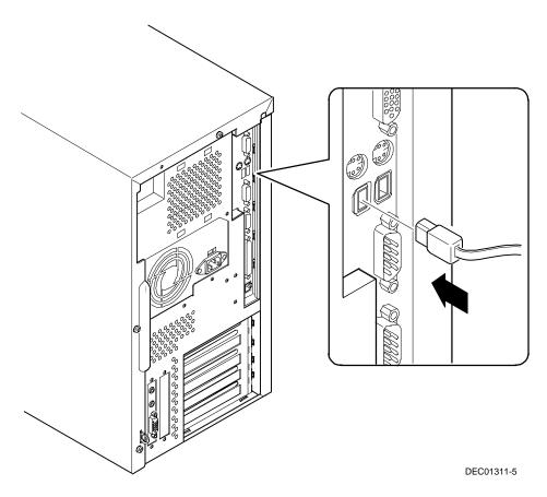
Figure 1-11. Connecting a USB Device
