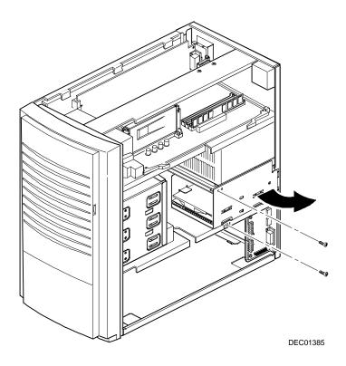
Figure 6-5. Accessing the Internal 31/2-Inch Device Bay
