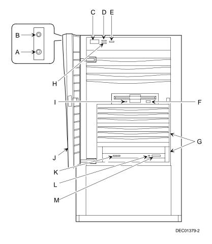
Figure 1-1. Front Panel Controls and Indicators
