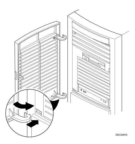
Figure 1-14. Replacing the Front Bezel Door
