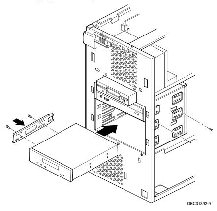
Figure 6-4. Installing 51/4-Inch Device
