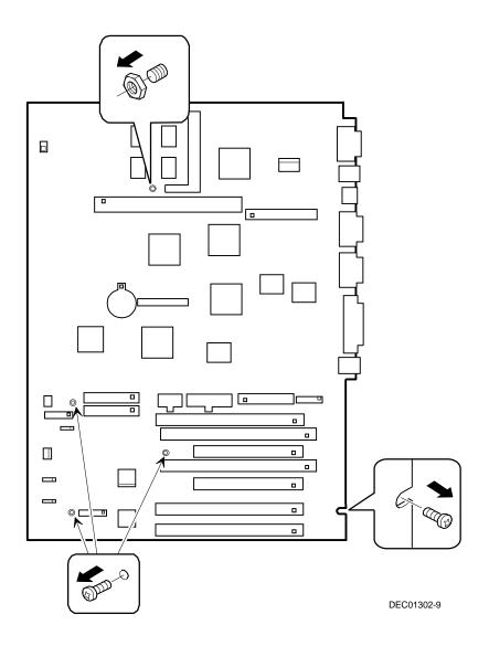
Figure 3-7. Removing the Main Logic Board
