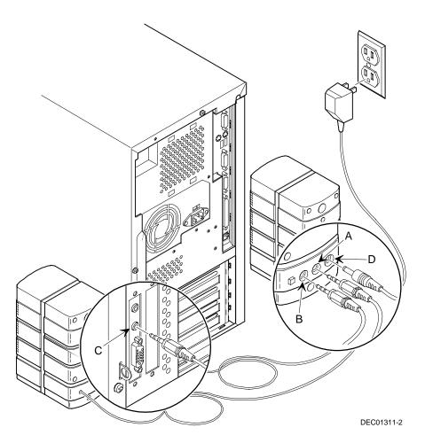
Figure 1-6. Connecting Speakers
