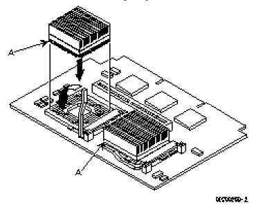
Figure 3. Installing a Second CPU Chip
