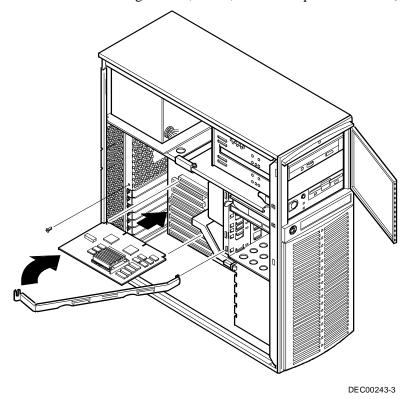
Figure 6. Installing the CPU Module
