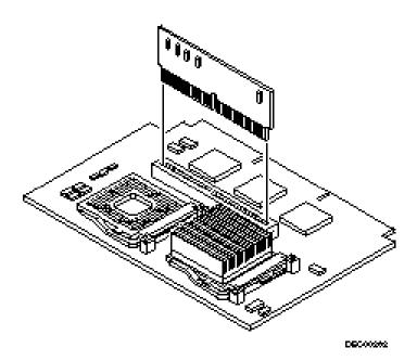
Figure 4. Installing the Secondary Cache
