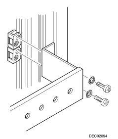
Figure 13: Align Bracket Assembly with Clips
