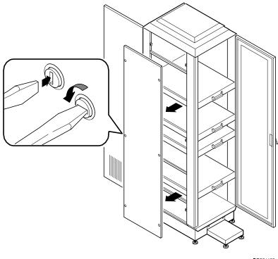
Figure 15: Reinstall the Side Panels
