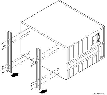
Figure 3: Installing the Server Mounting Brackets
