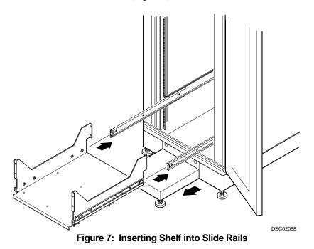
12. Attach the shelf to the slides by guiding the extended shelves into the shelf bracket (Figure 7).
