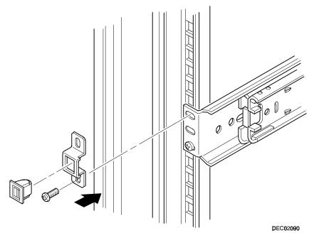
Figure 5: Installing Bezel Mounting Hardware
