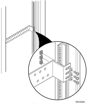
Figure 9: Installing Cable Management Bracket
