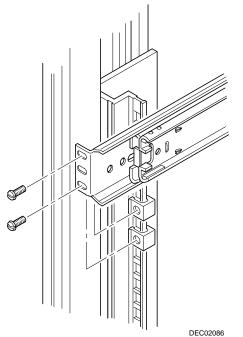
Figure 4: Adding Slides to Rackmount Rails
