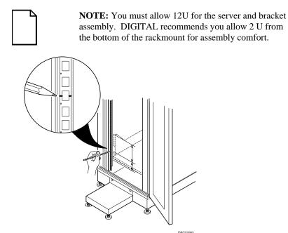
Figure 1: Marking the Installation Location
