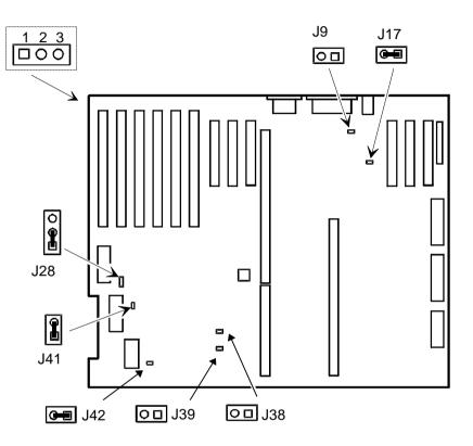
Figure 3 - 5 Main Board Jumper Locations
