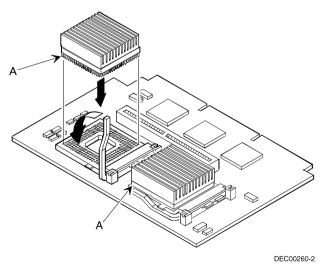
Figure 3 - 10 Replacing the CPU Chip
