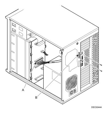
Figure 3 - 22 Connecting a external SCSI Bus
