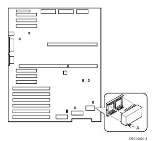
Figure 3 - 18 Replacing the Server Battery/Real Time Clock (RTC)
