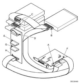
Figure 3 - 21 Connecting a Dual Channel SCSI Bus
