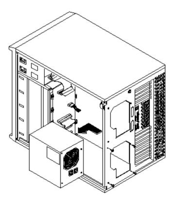
Figure 3 - 14 Removing the Power Supply
