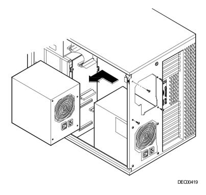
Figure 3 - 15 Removing the Optional Power Supply
