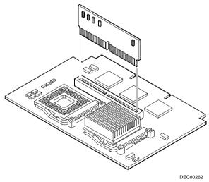
Figure 3 - 16 Replacing the Secondary Cache Module
