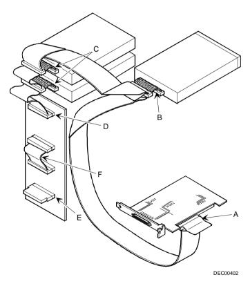
Figure 3 - 20 Connecting a Single Channel SCSI Bus
