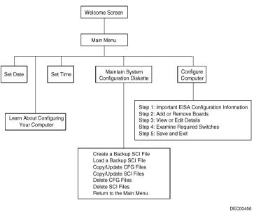
Figure 2 - 1 SCU Main Menu OptionsBefore Using the
