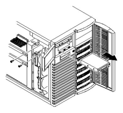
Figure 3 - 7 Replacing the 3½-inch Diskette Drive
