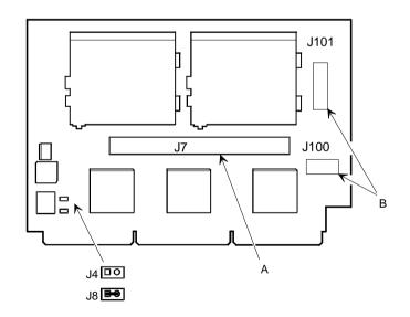
Figure 3 - 11 Set the CPU Voltage to 3.3 Volt
