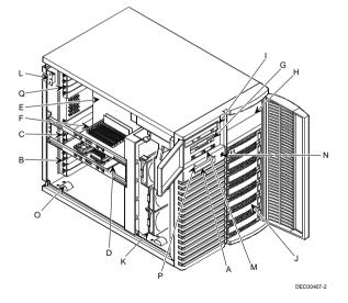
Figure 3 - 2 Server Components (Left Side)
