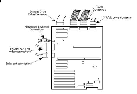
Figure 3 - 13 Removing the Main Logic Board
