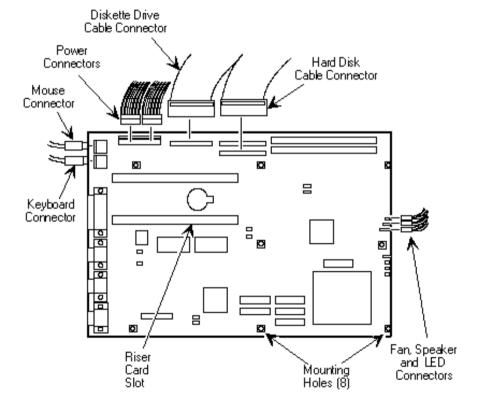
Figure 3 - 17 Removing the VENTURIS 486 Main Logic Board
