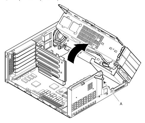
Figure 3 - 14 Opening the VENTURIS 486 Full-Profile Device Bay & Power Supply Subassembly
