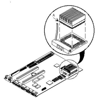
Figure 3 - 24 Installing a Higher Performance CPU on the VENTURIS 486 models
