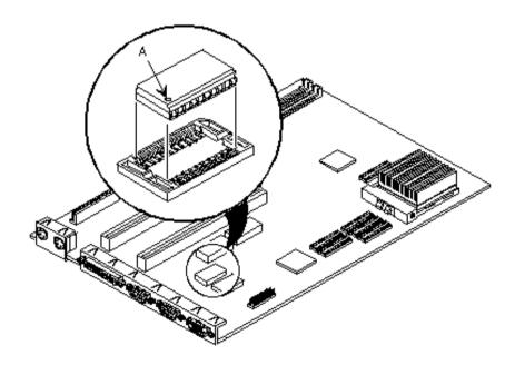
Figure 3 - 25 Installing Video Memory on the VENTURIS 486 Full Profile models
