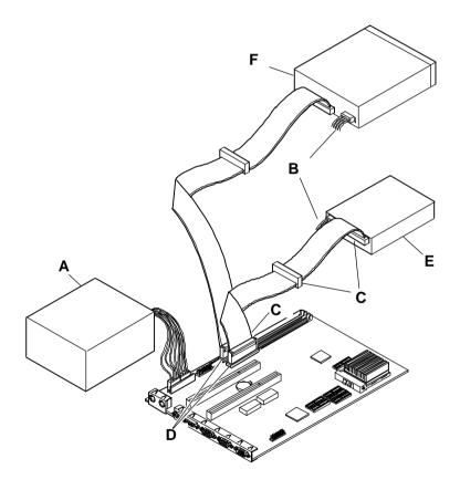
Figure 3 - 28 IDE Data Cable Connections
