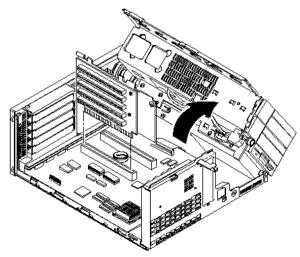
Figure 3 - 21 Removing the Riser Card & Bracket on the VENTURIS 486 Full-Profile models
