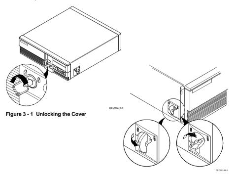
Figure 3 - 2 Releasing the Cover
