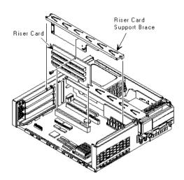
Figure 3 - 20 Removing the Riser Card & Bracket the VENTURIS 486 Slimline models
