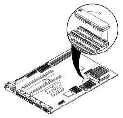
Figure 3 - 23 Installing External Cache Memory on the VENTURIS 486 version 2.0 board
