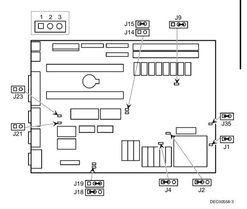
Figure 3 - 9 VENTURIS 486 version 2.0 Main Logic Board Jumpers Locations
