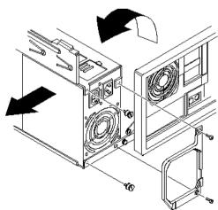
Figure 3 - 19 Removing the Power Supply on the VENTURIS 486 Full-Profile models
