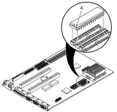
Figure 3 - 22 Installing External Cache Memory on VENTURIS 486 version 1.0 board
