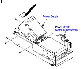
Figure 3 - 18 Removing the on Power Supply on the VENTURIS 486 Slimline models
