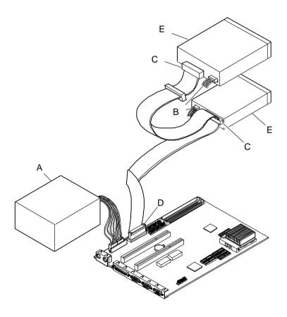
Figure 3 - 27 Diskette Data Cable Connections
