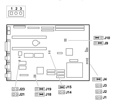
Figure 3 - 8 VENTURIS 486 version 1.0 Main Logic Board Jumpers Locations
