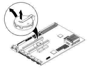
Figure 3 - 26 Replacing the Computer Battery on the VENTURIS 486 models
